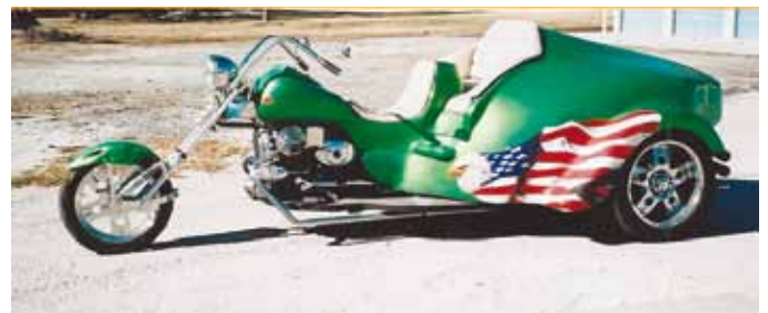
Jewel Ware Tells us his trike has a Honda front end and a front wheel drive Caddy V8 with auto trans. MO
